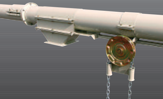
Intermediate outlet with longitudinal slide, chain operated
